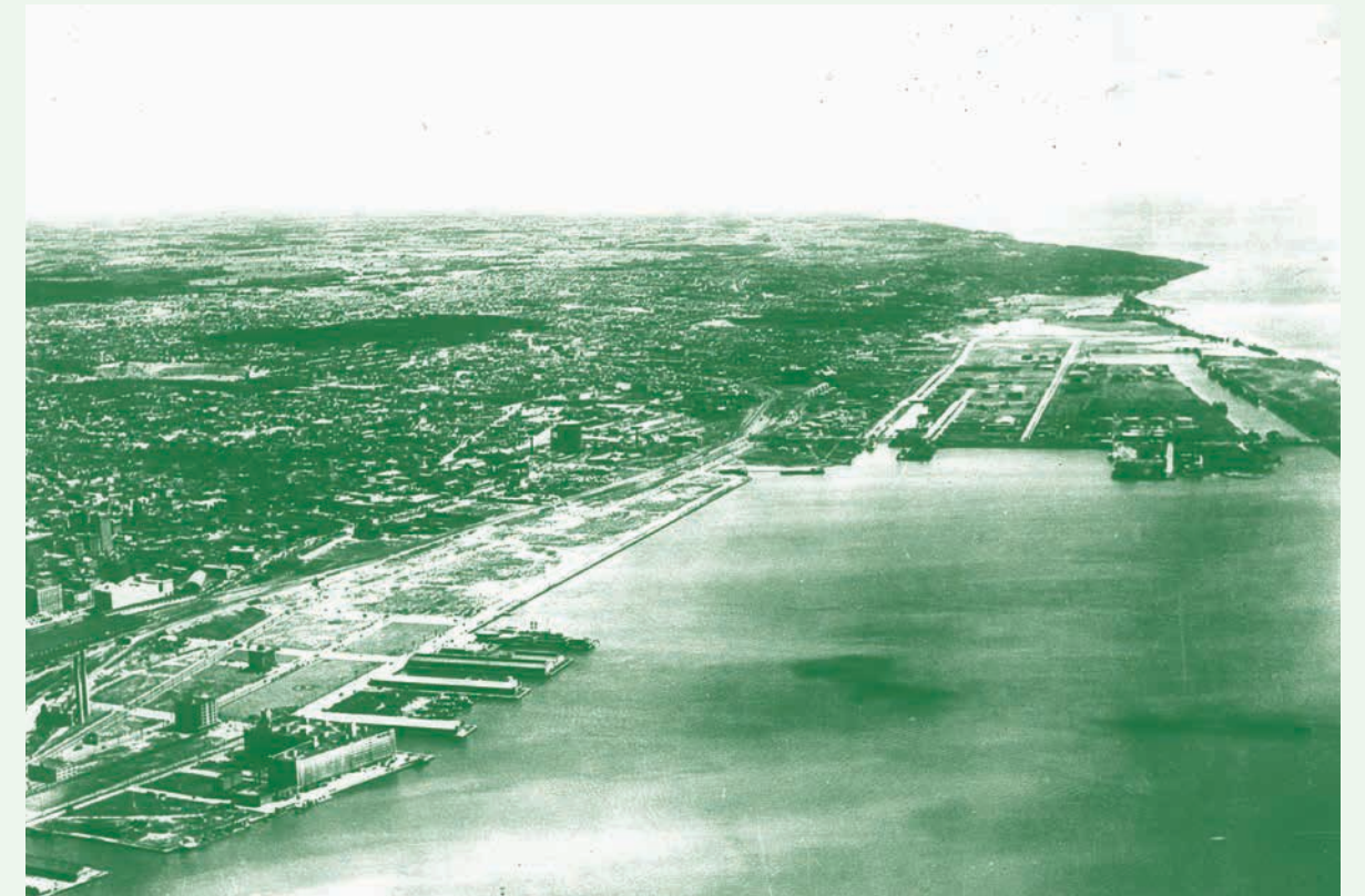
An aerial view of Toronto's waterfront looking east towards the Port Lands, from circa 1933, shows the industrial area created by filling in Ashbridge's Bay marsh. Credit: City of Toronto Archives
